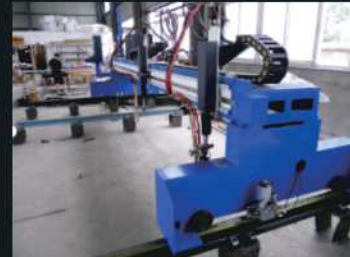
MODEL GCNC-FP GANTRY TYPE CNC PLATE & PIPE CUTTING MACHINE (OXY-FUEL / PLASMA)
