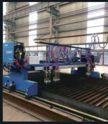
MODEL GMTS GANTRY TYPE MULTI-TORCH STRIP CUTTING MACHINE (OXY-FUEL)
