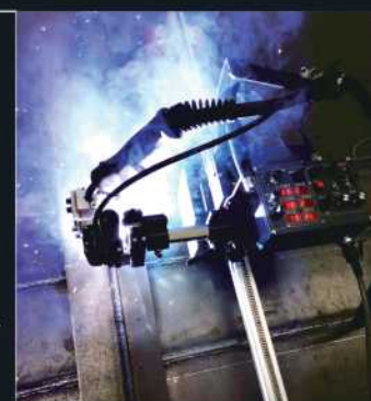
KC-72W2 with weaving unit & straight magnetic track
